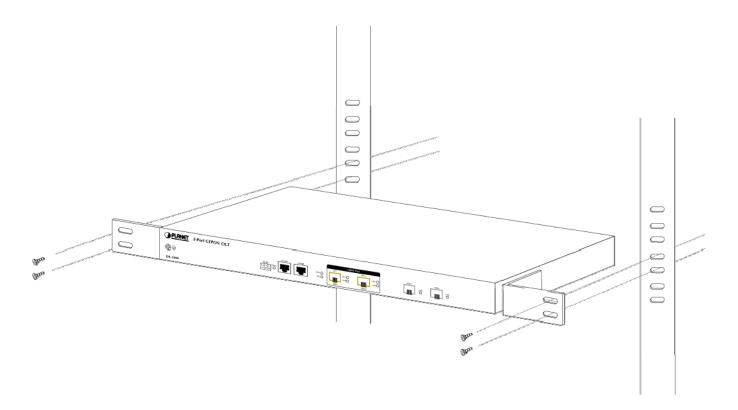
Figure 2-5 Mounting the GEPON OLT on a Rack
