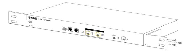
Figure 2-4 Attaching Brackets to the GEPON OLT.
