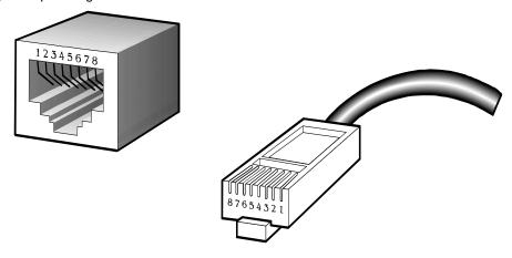
The standard RJ45 receptacle/connector
