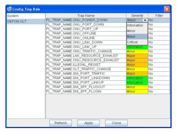
Figure 4-9 Config Trap Rule screen
