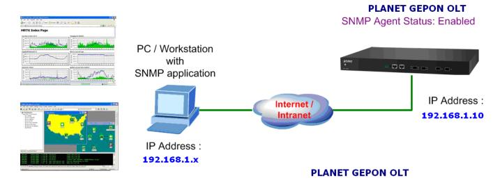
Figure 3-26 SNMP Management Diagram
